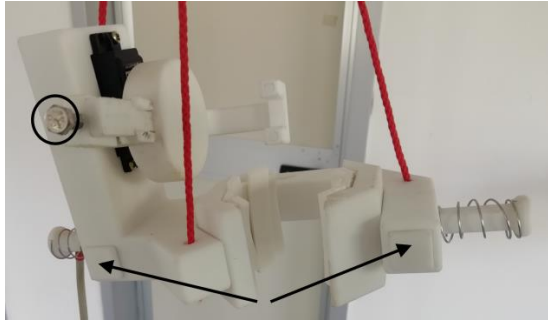
Fig. 13 The new clamp with ratchets, the arrows indicate the buttons to be pressed to release the ratchets, while the circle indicate the screw to set the proper position for the lever that guides the tip motion
