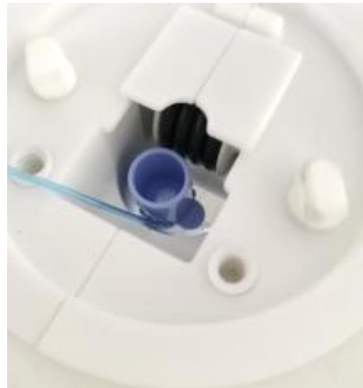
Fig. 12 Picture of the lower thrust element installed in ROSINA letting the connector of a cannula pass without problems
