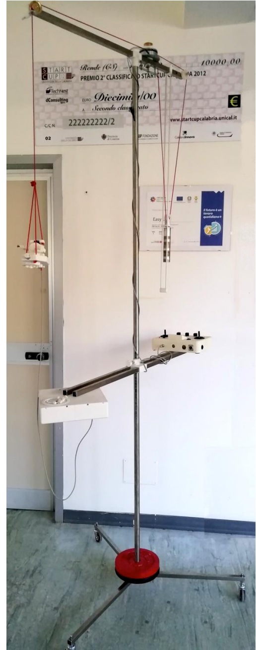
Fig. 8 The complete system built in the version with the motor mounted on the clamp
