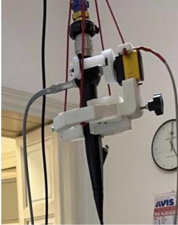
Fig. 7 The clamp to grasp the fiberscope suspending it on the vertical of the RA
