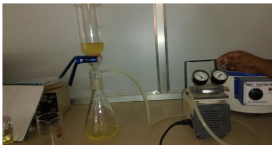
Fig 3 Positive pressure filtration unit used for the extraction of lycopene from the cake with acetone charges of 50 to 75 ml.
